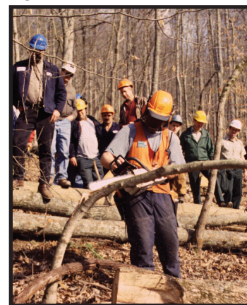
Figure 2. Small spring pole being cut by a Kentucky Master Logger chainsaw instructor. Spring poles can be much bigger.
